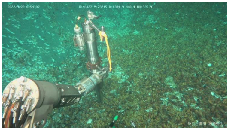
Figure 3-1-42 The deep-sea sediment (natural gas hydrate) coring system with temperature and pressure preservation in operation
